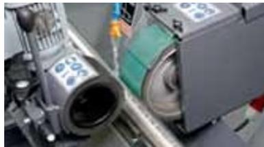
Optimum grinding of welded seams. Perfect satin-finishing and polishing for pipe bends
